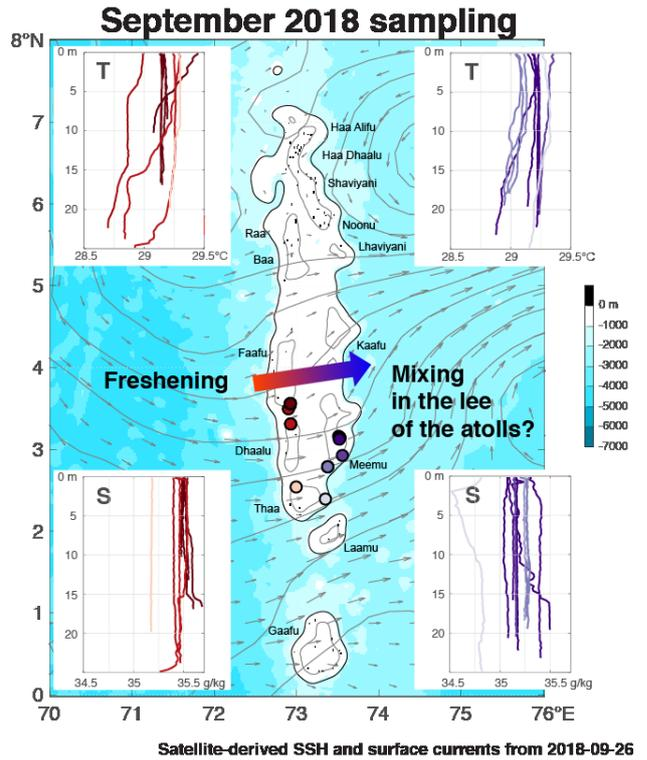
CTD data overlapped on a map showing the currents at the surface estimated from satellite. West side data is in red, east side is in purple. Temperature is plotted on the top panels, salinity on the bottom ones.
